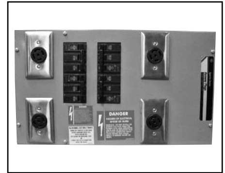
Spectra Series twist lock plug Equipped with plug assist, 30-150A, 208/120V, 22kAIC Plugs directly on Spectra Series busway Compact design 20.25" L x 11.66" W x 5.15" D
