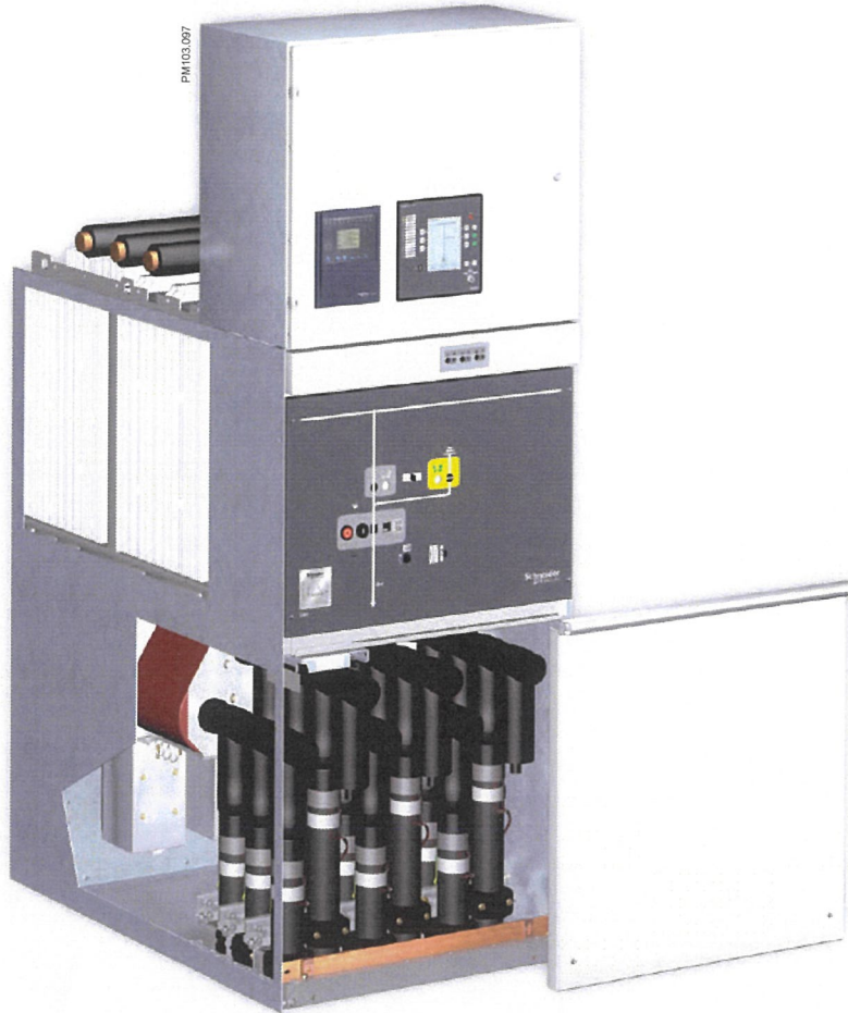
800 mm switchgear cubicle, equipped with voltage transformer, 4 cables/conductors (double cone) and surge arrester Illustration: up to 2000 A
