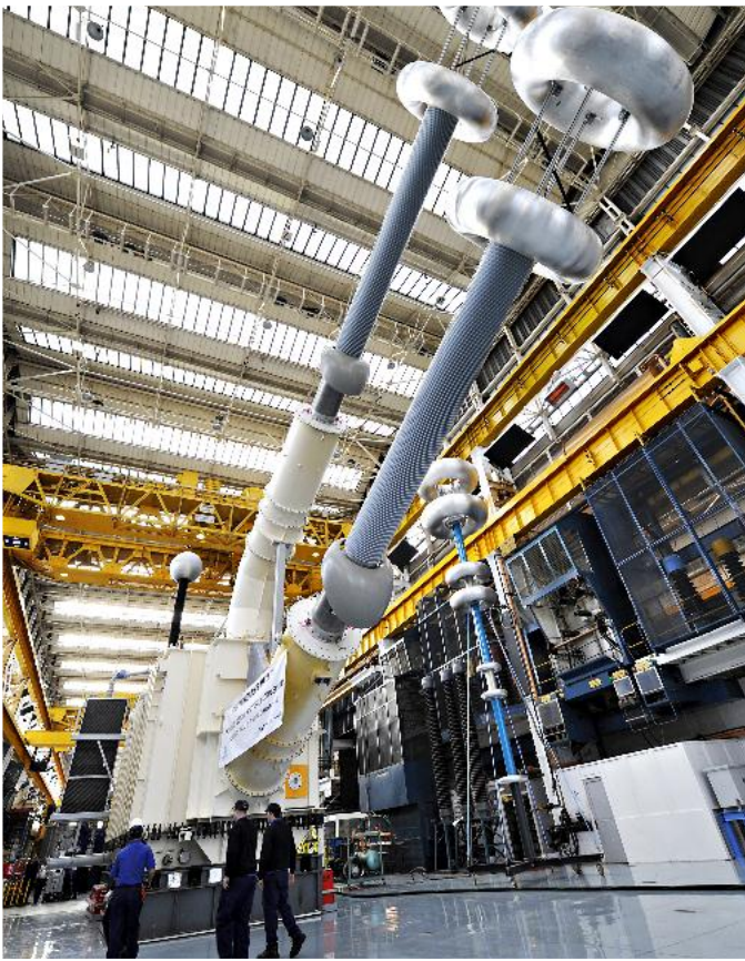
HVDC converter transformer 600 kV DC for Rio Madeira, Brazil
