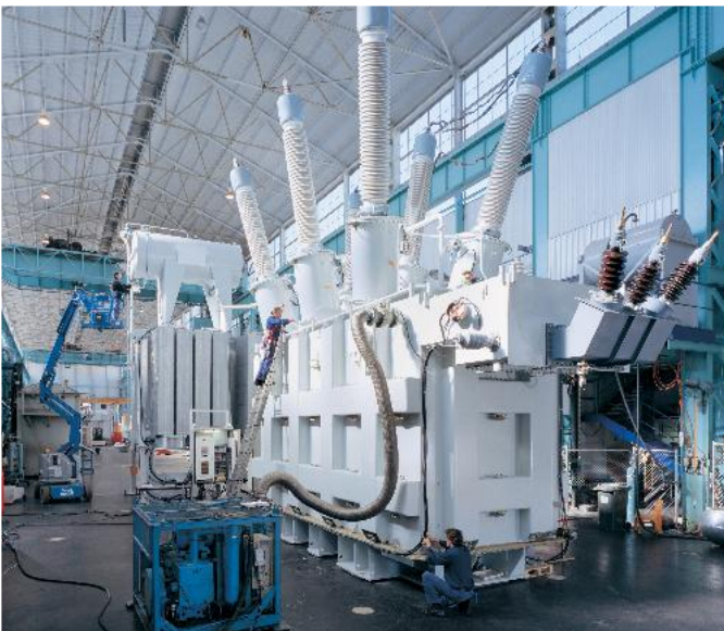
Manufacturing of a 1125 MVA 330/275/33 kV autotransformer for Middle Ridge s/s (Australia)
